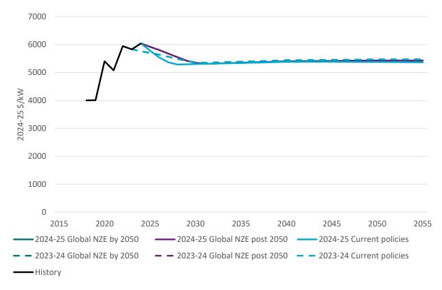
Figure 5-3 Projected capital costs for black coal ultra-supercritical by scenario compared to 2023-24 projections
