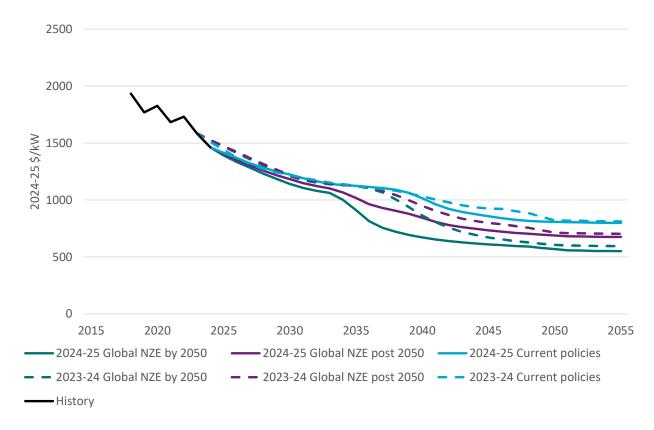
Figure 5-11 Projected capital costs for large-scale solar PV by scenario compared to 2023-24 projections
