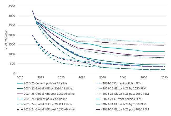
Figure 5-20 Projected technology capital costs for alkaline and PEM electrolysers by scenario, compared to 2023-24
