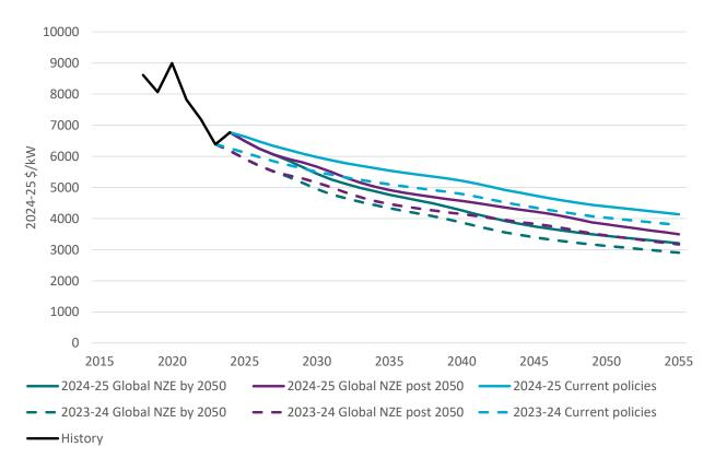
Figure 5-10 Projected capital costs for solar thermal with 14 hours storage compared to 2023-24 projections
