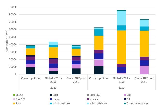
Figure 5-1 Projected global electricity generation mix in 2030 and 2050 by scenario The technology categories displayed are more aggregated than in the model to improve clarity. Solar includes solar thermal and solar photovoltaics.
