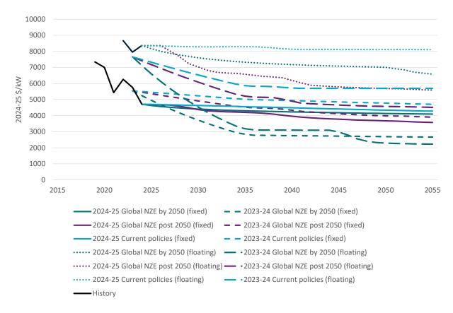
Figure 5-14 Projected capital costs for fixed and floating offshore wind by scenario compared to 2023-24 projections
