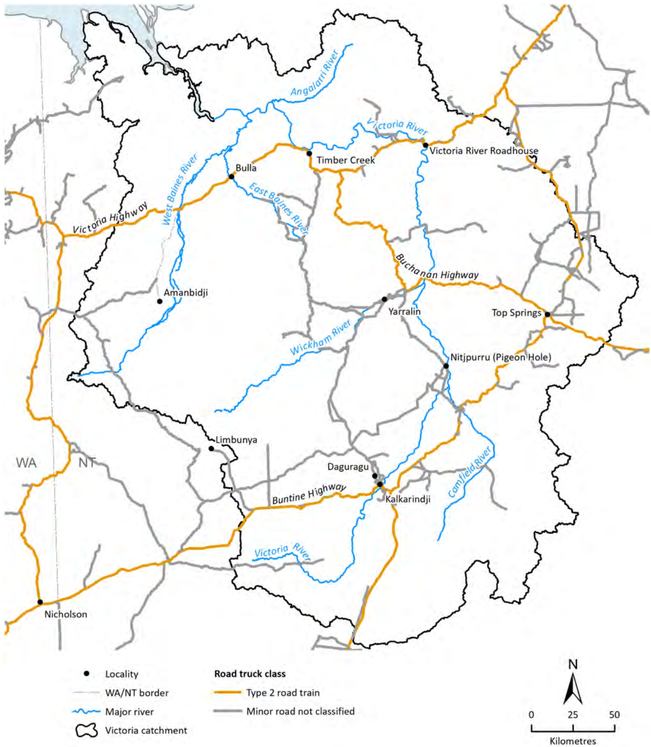
Figure 3-14 Roads accessible to Type 2 vehicles across the Victoria catchment: minor roads are not classified Type 2 vehicles are illustrated in Figure 3-15.
