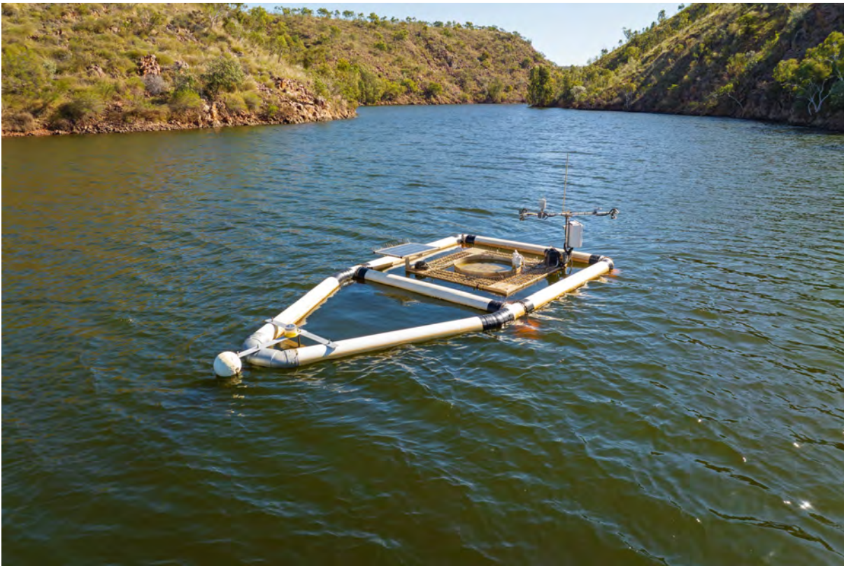
Figure 3-1 Floating evaporation pan used to determine water surface evaporation, Lake Julius on the Leichhardt River
