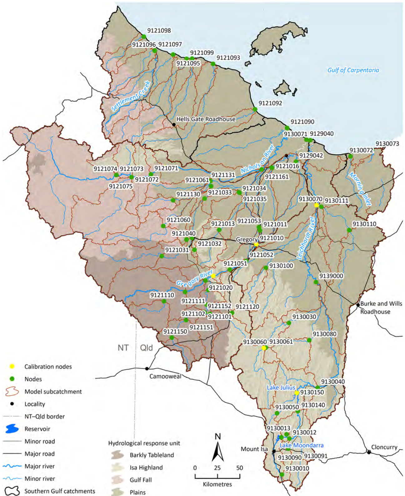
Figure 5-1 River model nodes and subcatchment areas. Hydrological response units are based on physiographic units identified for the region
