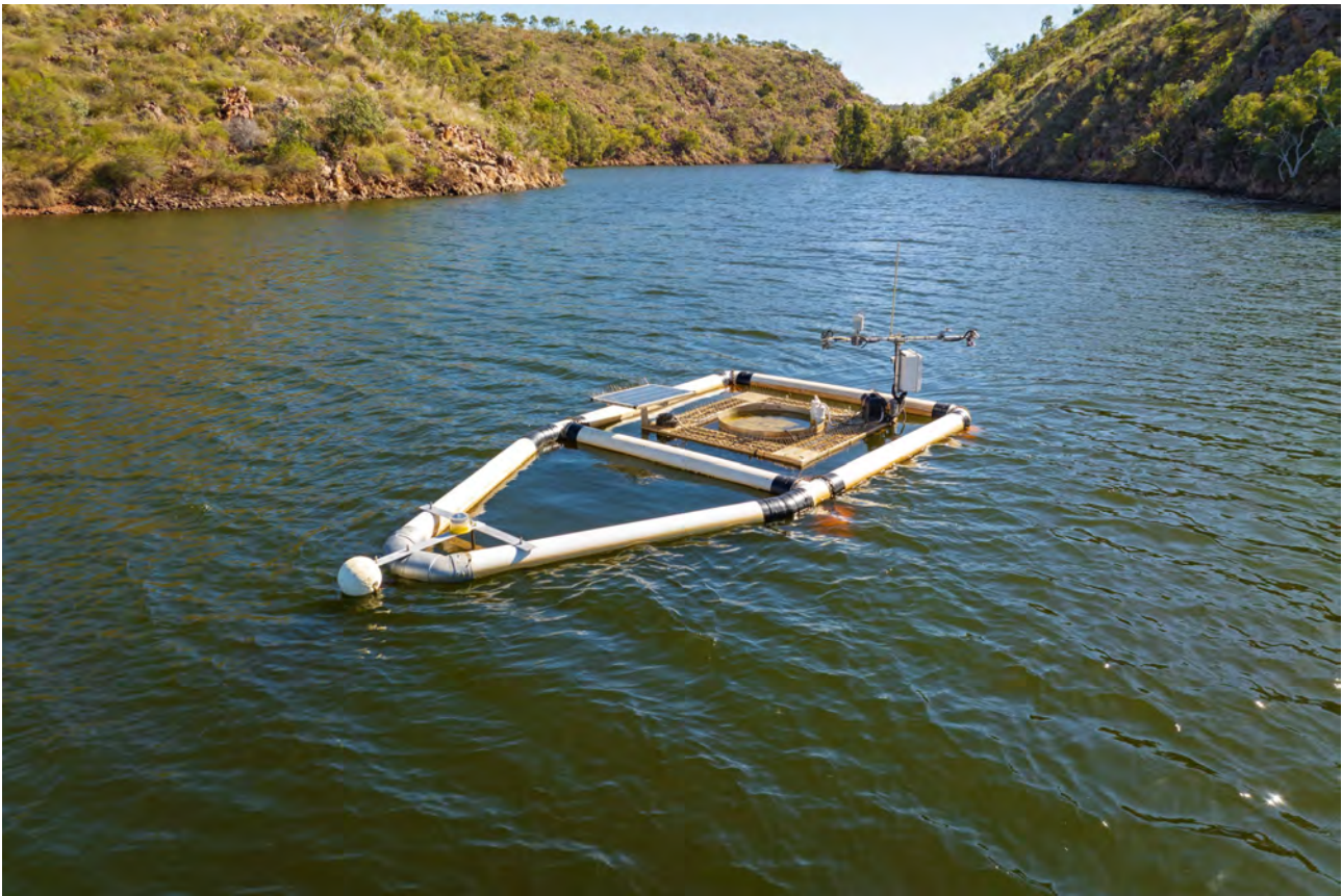
Figure 4-1 Floating evaporation pan used to determine water surface evaporation, pictured on Lake Julius on the Leichhardt River
