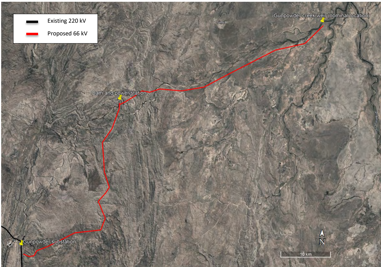
Figure 3-3 Concept of connection route from the Gunpowder Creek weir to the 220 kV transmission line for Option B
