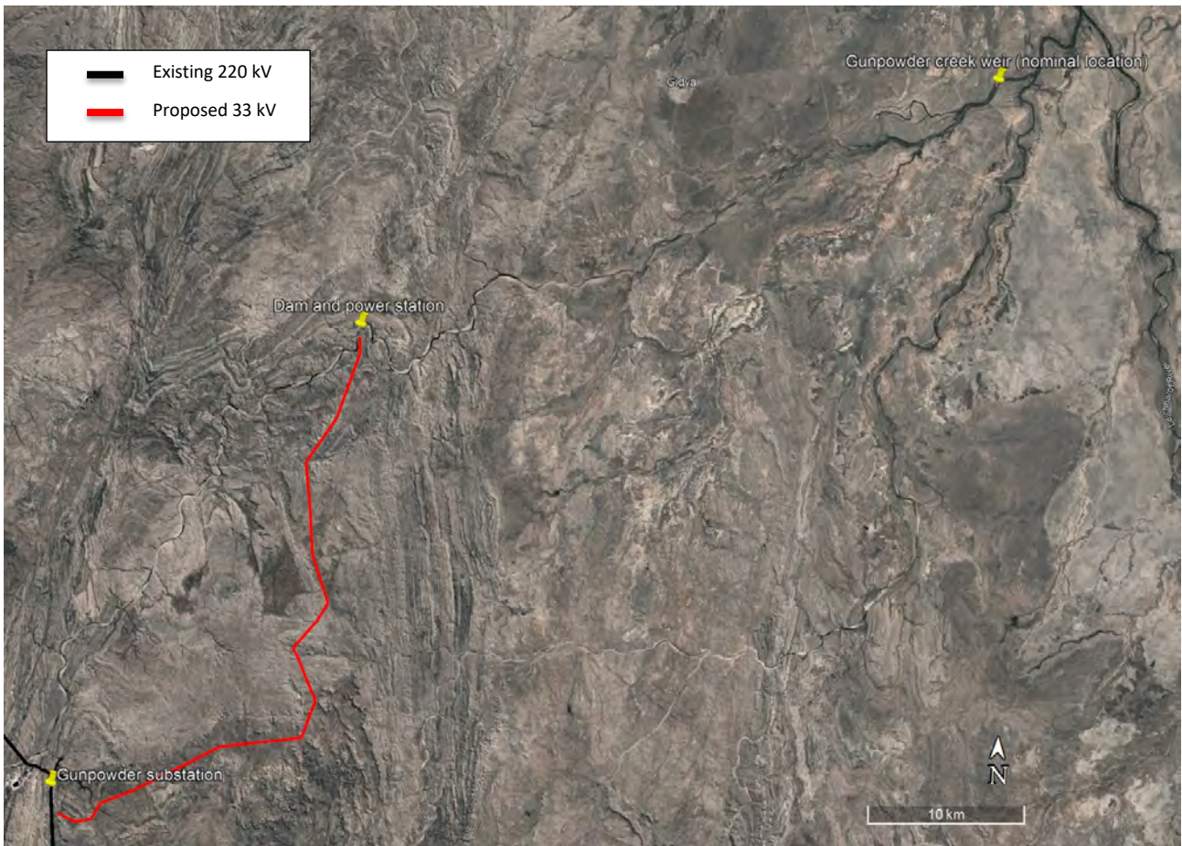
Figure 3-2 Concept of connection route from the dam and power station to the 220 kV transmission line for Option A
