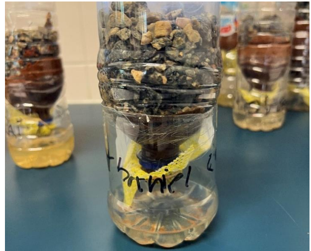
Figure 1: Student water filters using stones and sand. Teacher: Rebecca Mackin, Onslow Primary School. Photo: David Broun CSIRO.
