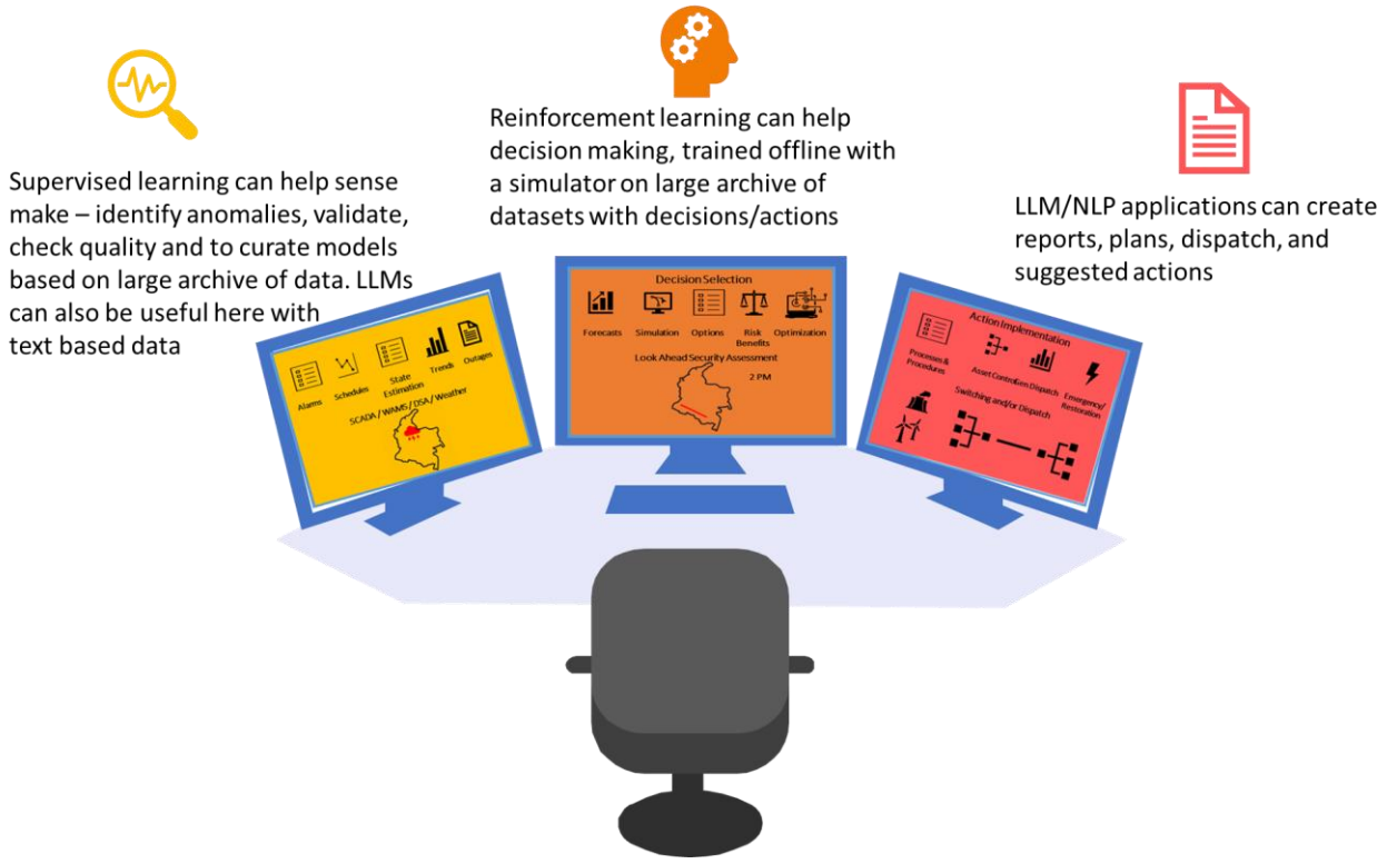
Figure 37 The classes of AI/ML that can support the operator in the controls room in their three modes of operation.
