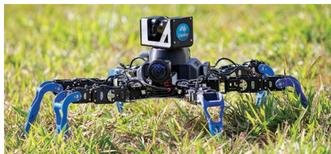
Zee: prototype hexapod robot equipped with a streaming camera sensor and a real-time 3D scanning LIDAR.
