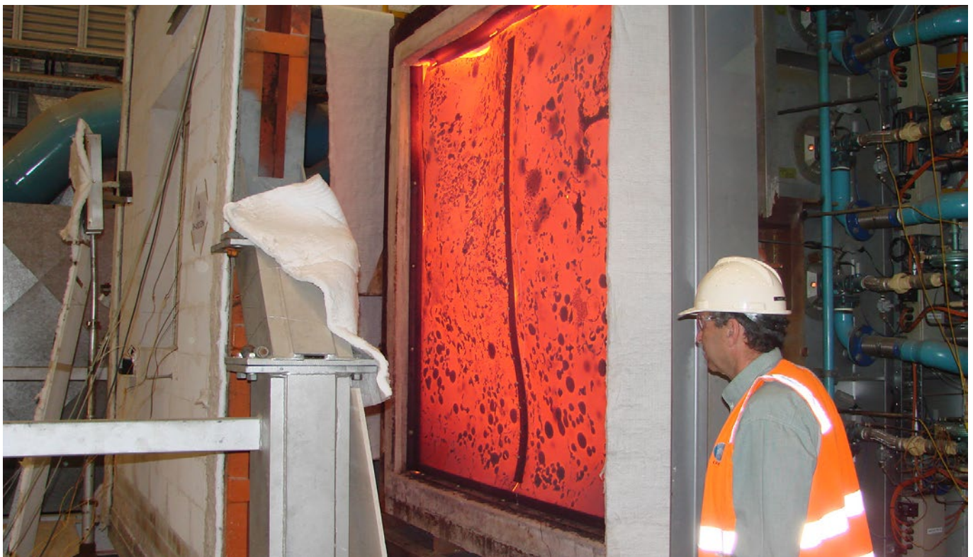
Large scale AS1530.8 test for buildings exposed to bushfire attack (radiant heat) at CSIRO, North Ryde site, NSW.
