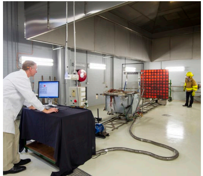
Testing on a small scale for radiant heat exposure for building materials. CSIRO, Clayton site, Victoria.
