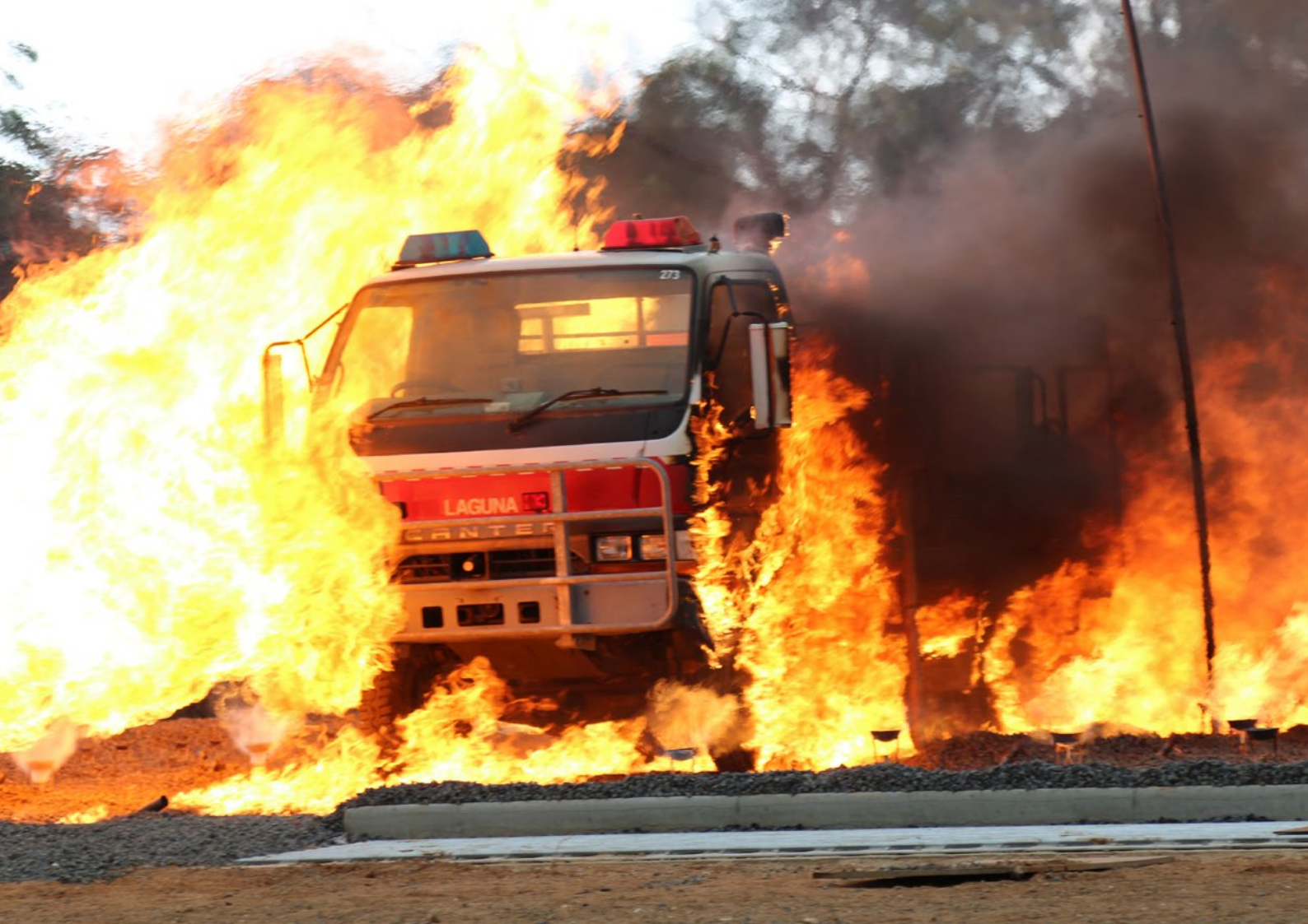
CSIRO testing of firefighting vehicles to support development of crew protection systems.
