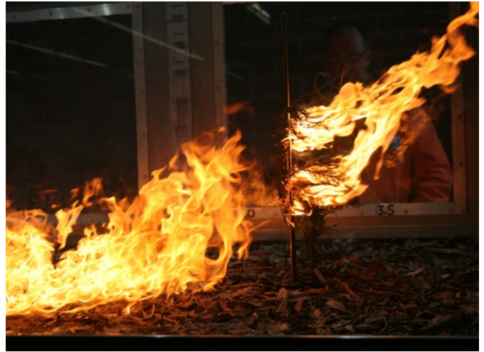
Experimental fire in CSIRO's Pyrotron. Scientists study ignition shrub fuels from surface fire.
